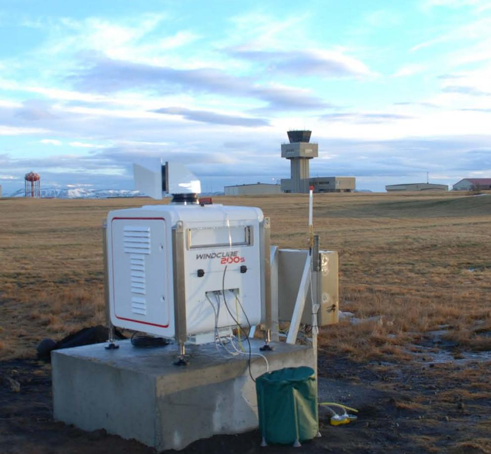
Lidar (also written LIDAR, LiDAR or LADAR) is a surveying technology that measures distance by illuminating a target with a laser light.
